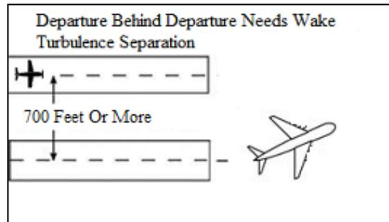
**h.** Separate aircraft departing from a parallel runway separated by 2,500 feet or more if projected flight paths will cross (See FIG 3-9-8):
